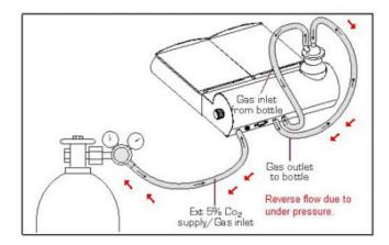
The fault occurs because of under pressure in the gas supply when the G85 is not in use.
