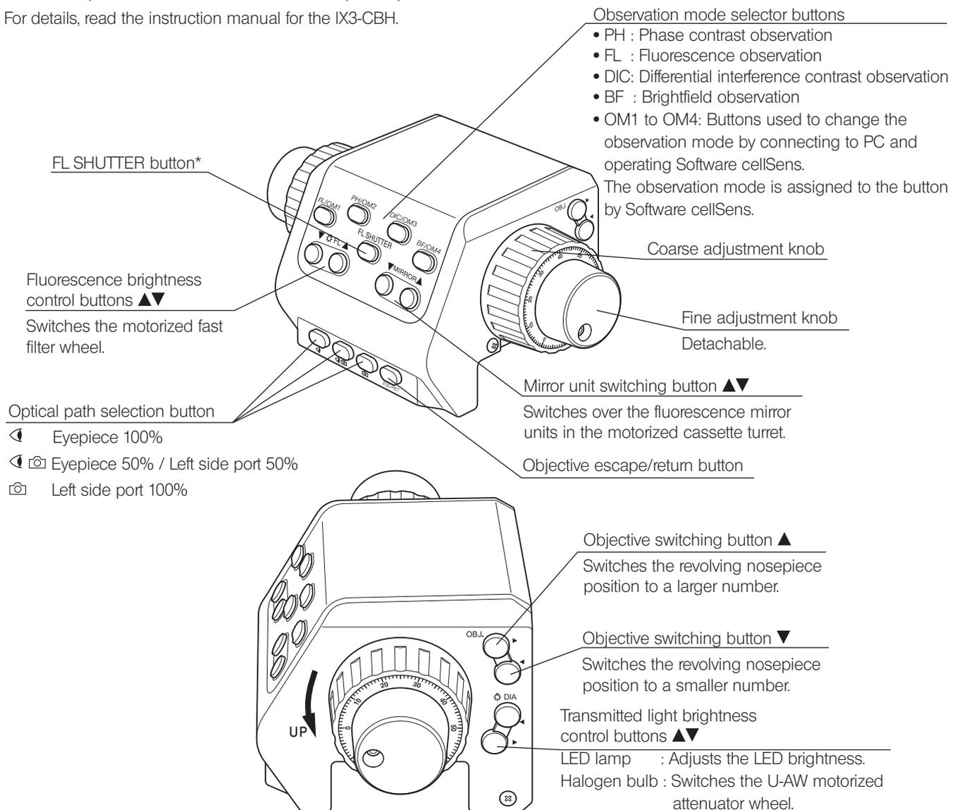
\* The FL SHUTTER button opens/closes the reflected shutter only. The transmitted shutter opens/closes automatically depending on the observation modes.
