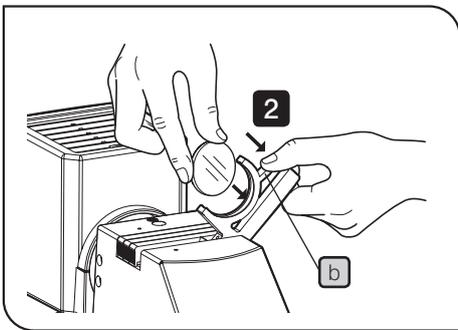
**2** While holding the mounting lever **b** of the filter holder, insert a filter.
