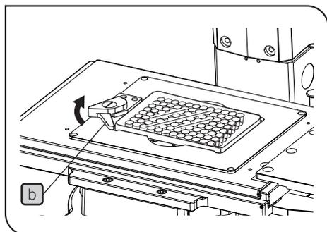
Open the specimen holder **b** of IX3-HOW, set the microplate in the center, push it toward the right diagonal direction, and return the specimen holder back to the original position.
