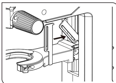
**CAUTION** If the condenser refocusing stopper is attached when the condenser attaching arm is placed at the lower position, the condenser may not be attached. Be sure to raise the condenser attaching arm before attaching the condenser refocusing stopper.
