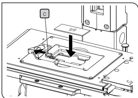
Open the specimen fixing part **c** of IX3-HOS outward, set the specimen in the center, push it toward the right diagonal direction, and return the specimen fixing part back to the original position.
