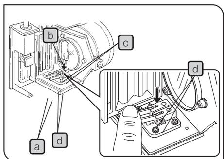
**CAUTION** To prevent reduced bulb life or cracking, do not touch the bulb with bare hands. If fingerprints are accidentally left on the bulb, wipe the bulb with a dry soft cloth.
