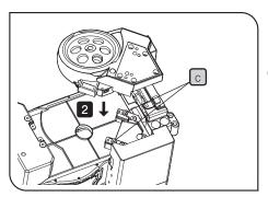
2 Insert the revolving nosepiece slowly into the positioning pins © (2 positions) in the upper area of the microscope.
