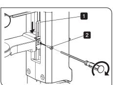
If the condenser refocusing stopper is attached when the condenser attaching arm is placed at the lower position, the condenser may not be attached. Be sure to raise the condenser attaching arm before attaching the condenser refocusing stopper.
