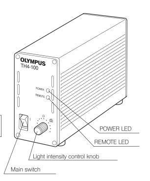
The applicable halogen bulb is the 12V100WHAL-L For details, refer to the separate instruction manual.
