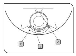
The attaching method is identical to that for the phase contrast optical elements (page 34), except that the positioning pin and positioning groove should be aligned when attaching each DIC optical element.
