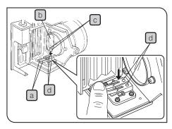
To prevent reduced bulb life or cracking, do not touch the bulb with bare hands. If fingerprints are accidentally left on the bulb, wipe the bulb with a dry soft cloth.
