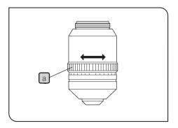
If the thickness of the cover glass or the vessel does not match the thickness scale of an objective with correction collar, the objective cannot manifest its performance. When using a correction collar equipped objective, perform the following adjustment as required.
