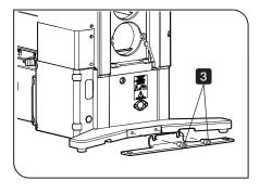
3 Attach the fixing plate on the back side of the microscope and fix it by using the commercially available 5 mm Allen wrench.
