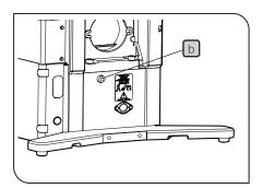
Releasing the transport lock of the light path selector
