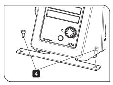
4 Tighten the fixing screw by using the commercially available 5 mm Allen wrench to secure the microscope on the anti-vibration table.
