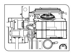
Put the cables coming from the modules attached to 1st Deck and 2nd Deck through the cable cover as shown in the picture on the left.
