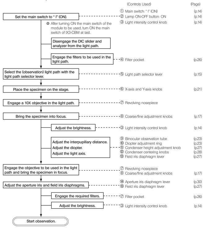
When you turn OFF the power, turn OFF the main switch of IX3-CBM first and then turn OFF the main switch of the other modules.7
