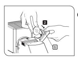
2 While holding the mounting lever b of the filter holder, insert a filter.
