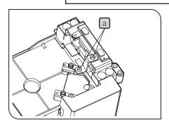
Releasing the transport lock of the focusing mechanism
