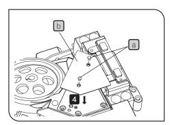
4 Place the cover b over the revolving nosepiece, and tighten the cover fixing screws a (2 positions) by using the Phillips screwdriver.
