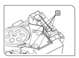
3 Tighten the revolving nosepiece fixing screws d (5 positions) by using the Allen wrench provided with the microscope.
