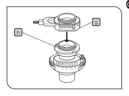
The polarizer can be mounted only on the IX2-LWUCD.
