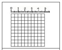
**Figure 2:** Schematic drawing of the view of the stage micrometer through the reticle.
