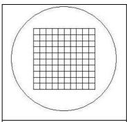
Figure 1: Schematic drawing of the view through the eyepiece with reticle.
